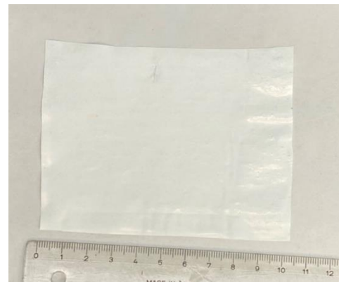
Figure 10. Preparation process and photograph of the LATP/PVdF-TrFE hybrid membranes.
